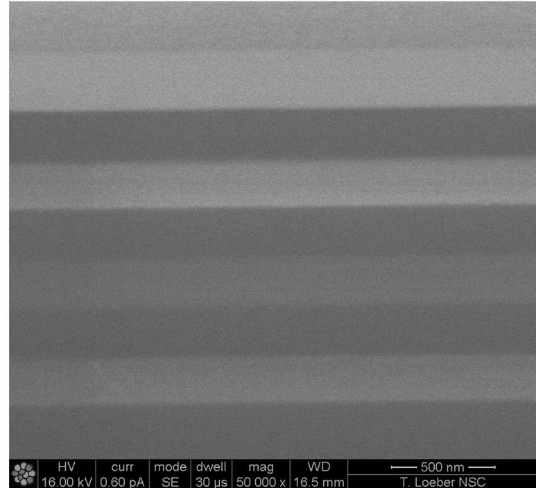
GaAs/AlGaAs layer: higher Ga beam better contrast, destroying cross section
