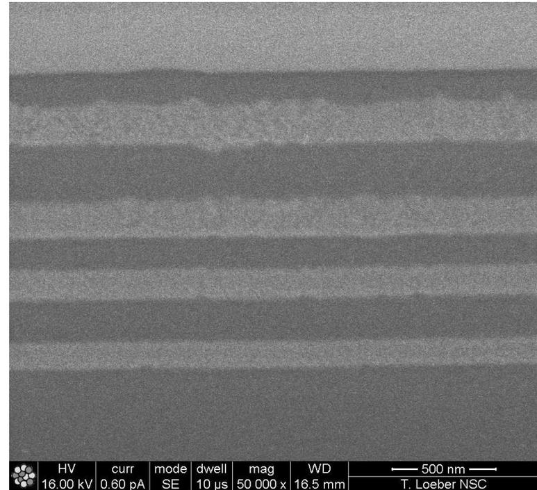
cross section done with Ga: not “clean”, dots, layers damaged
