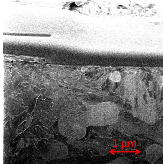
unpolished cross section of a piece of steel: 100Cr6
