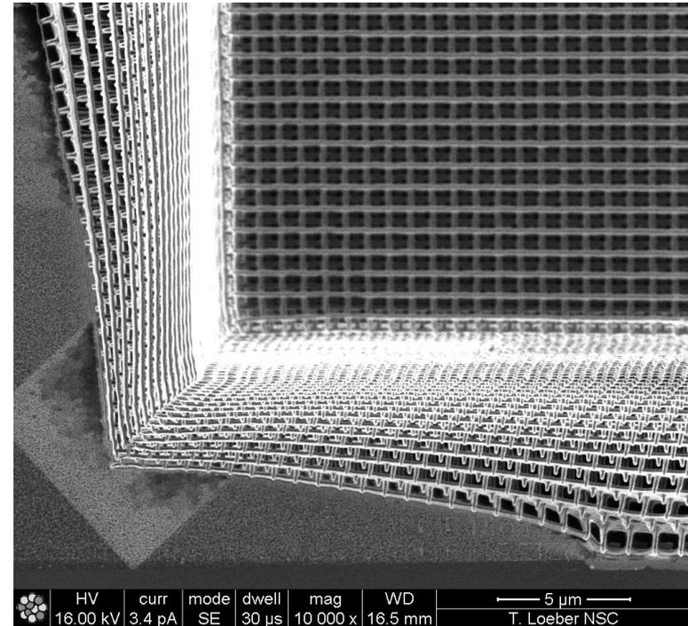
wood pile height 120 μm
