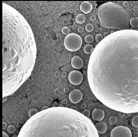
Tin Spheres 10  $\mu\text{m}$  FOV
