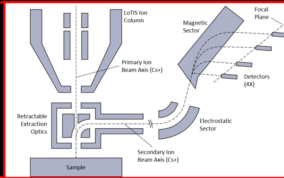
Single-Beam FIB with high-efficiency collection of secondary ions
